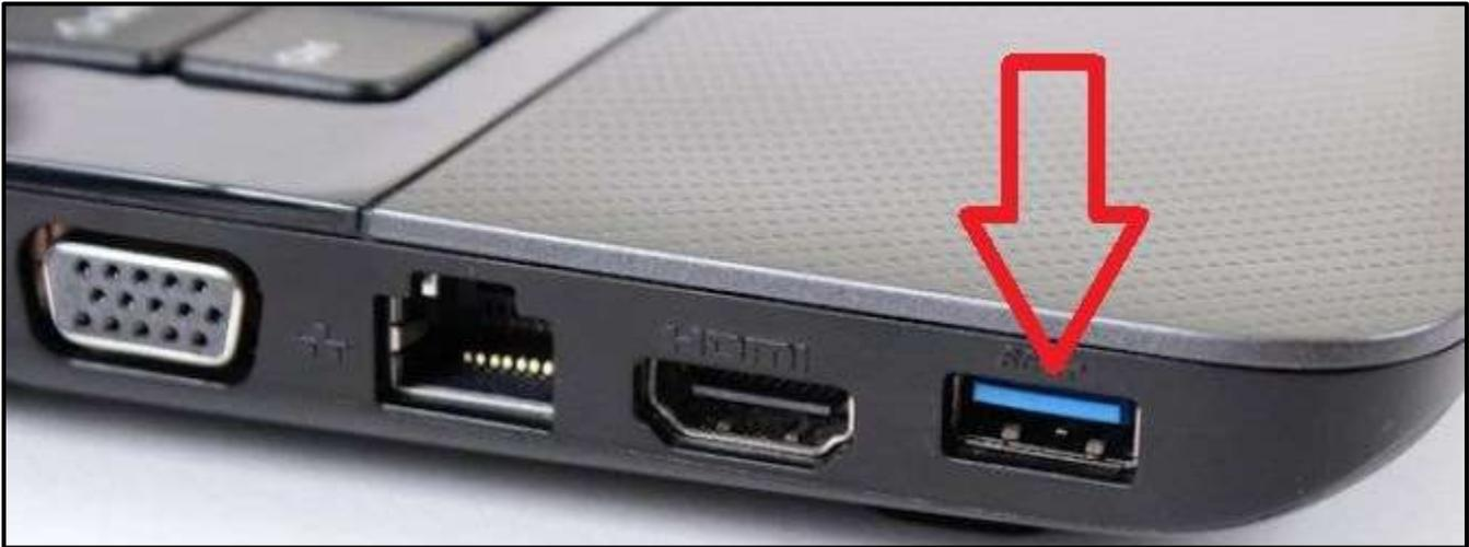
You might have to un-plug other devices to find a blue USB 3.x port. Using a black or white USB port does NOT meet the minimum requirements for SDFI. SDFI needs the use of a blue USB 3.x port to work right. Connect the blue end of your SDFI Card Reader into a Blue USB 3.x port on your computer. (A Blue port means it is fast and that it is USB 3.x)
